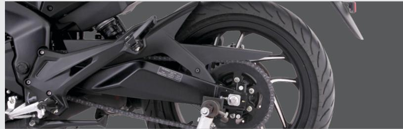
Ensure application of 9 to 11 Kgf.m torque to rear axle nut.
