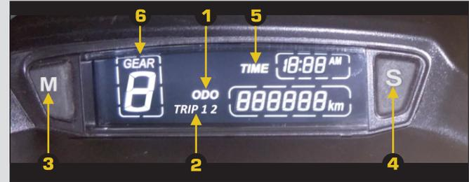
1. **Odometer** : The Odometer shows the total distance that the vehicle has covered. Odometer can not be reset to 'Zero'. Range 0 to 9.99.999 km.
