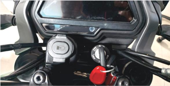
Mobile charging socket is provided near Ignition switch as an OE fitment.
