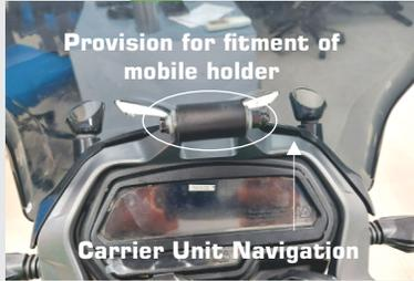
Provision for fitment of mobile holder a carrier unit navigation is provided above speedometer as an OE fitment.
