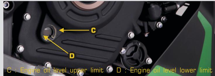
C : Engine oil level upper limit    D : Engine oil level lower limit
