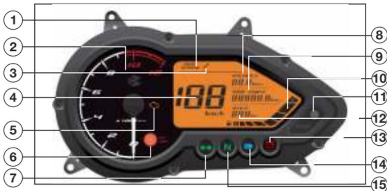
8. **IFE/AFE** : It display instantaneous / average fuel economy in km/l. at any given time. Value will be displayed in vehicle speed & engine RPM is more than zero.
