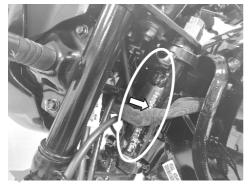
Frame Number Location On Side of Steering Tube (Alpha-Numeric - 17 Digits)
