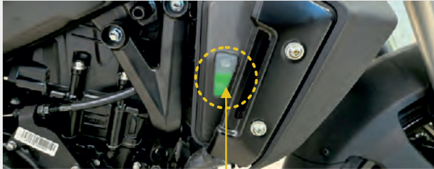
Coolant Expansion Tank
