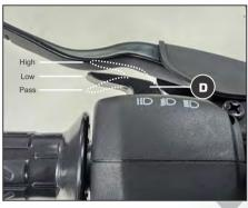
**D. Pass Switch:** Press the switch to put 'ON' Hi Beam/ Low Beam/ Pass light.
