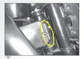
**Frame Number Location**On RH Side of Steering Tube (Alpha-Numeric - 17 Digits)
