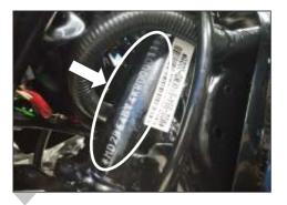
**Frame Number Location**On Side of Steering Tube (Alpha-Numeric - 17 Digits)
