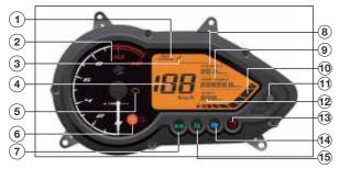
Side Stand Indicator: It glows when Side stand is down & igntion switch is 'ON' and kill switch in 'Engine ON' position.
