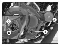
A: Oil Filler Cap, B: Oil Level Gauge
